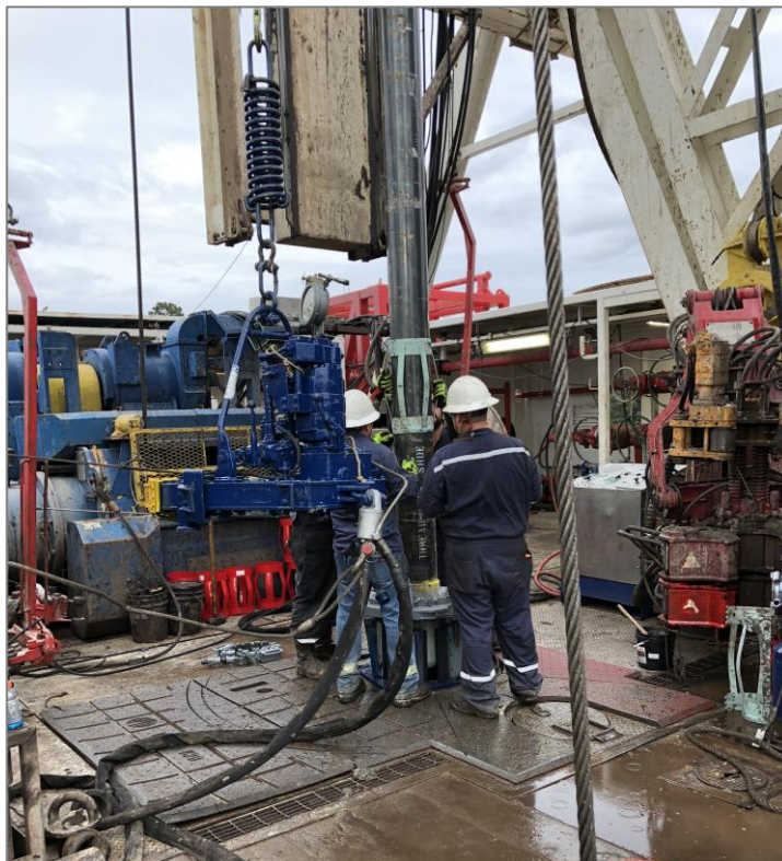
Running casing for the Stewart 30H-1
